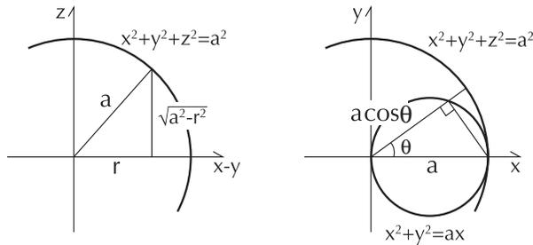
$$\frac{1}{2}V = \iint_{(x-\frac{a}{2})^2+y^2 \leq \frac{a^2}{4}} \sqrt{a^2 - x^2 - y^2} dx dy$$
